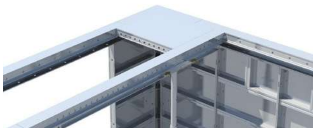
4. Installation of end beams (EB) and middle beams (MB)
