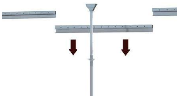
4. Dismantlement of soffit length
